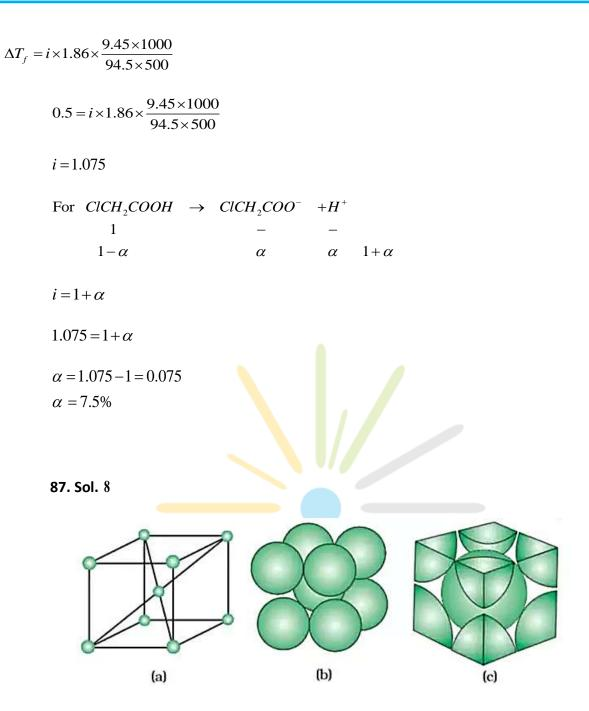
A body centre unit cell has 8 atoms at the corners of the unit cell and one atom at the body centre of the unit cell making the coordination number 8.
