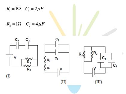
The time constants (in  $\mu S$ ) for the circuits I, II, III are respectively
